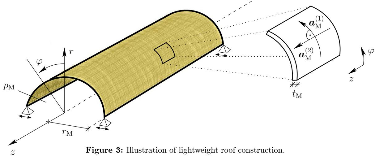
**Figure 3:** Illustration of lightweight roof construction.
